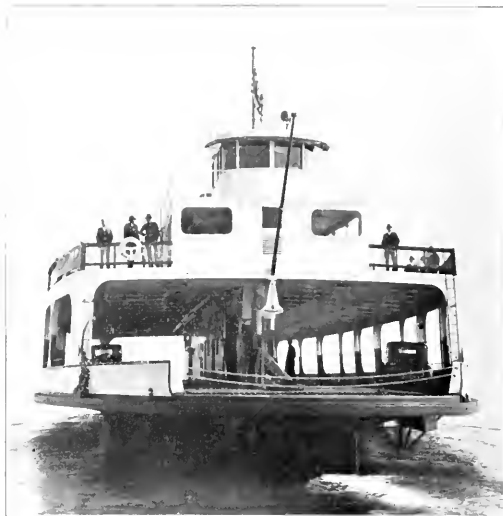
End view of the San Diego showing narrow engine room casing, leaving wide deck available for vehicles.
